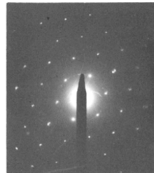
Figure 4 Clay mineral lamella extracted by carbon replica and its diffraction pattern.
